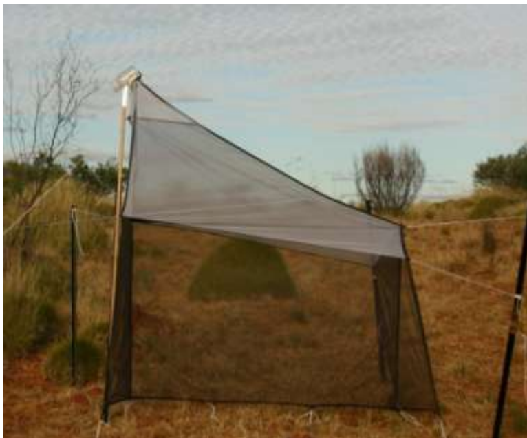
A sophisticated flight intercept trap called a Malaise trap. The insects fly into the dark mesh and move up towards the light mesh which eventually tapers to a collection container seen at the top left.
